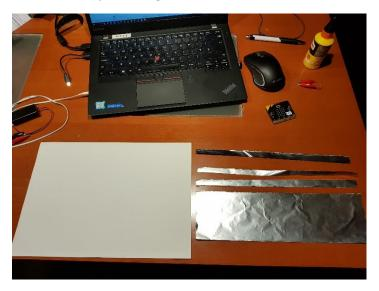
3. Glue the tin foil strips to the paper. Leave few millimetres between them. The thick foil should cross the fold.
