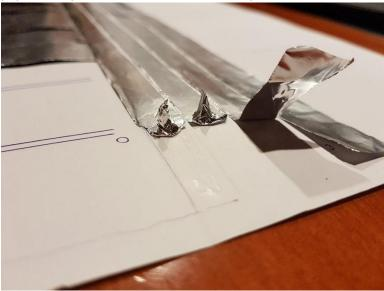
5. Fold the paper and cut the keys.Glue paper on the thin tin foil strips under every key as it is shown on the picture below. This way each key will get a unique code. Code 000 is silence.
