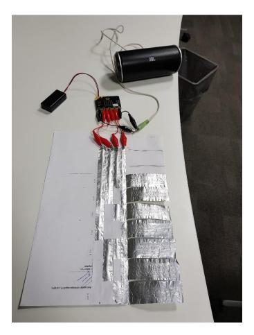
6. Connect the microbit to the paper piano and to the headset.
